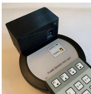
Hold the Test Unit as still as possible at a distance of approximately 50-70cm (c.1-2¼ ft) from the detector, close to the centre of the detector's line of sight, taking care to point the Test Unit emitter towards the detector's sensors.
