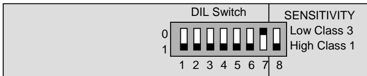
Fig 5 DIL Switch with Detector Front Cover Removed (Normal factory settings shown)
