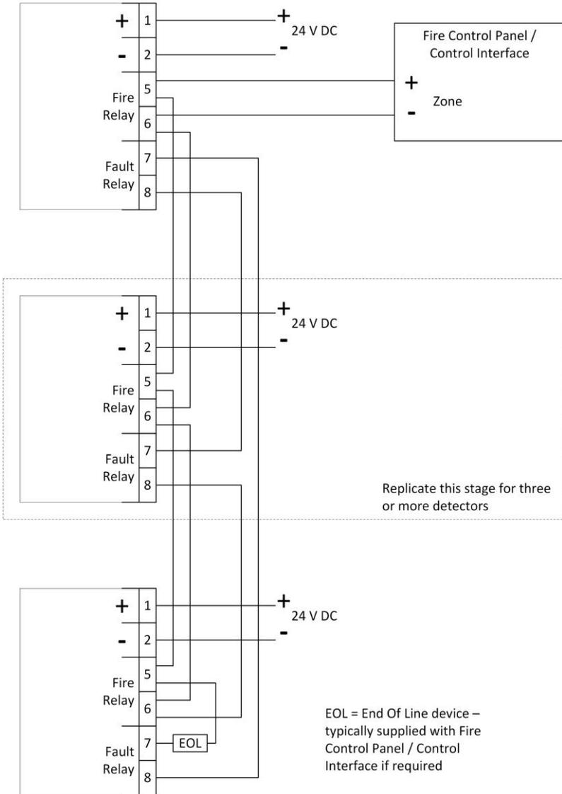
**Fig 7b** 4 Wire Connection Diagram – multiple detectors
