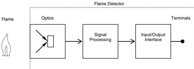
**Fig 7** Block Diagram of the Detector Signal Processing
