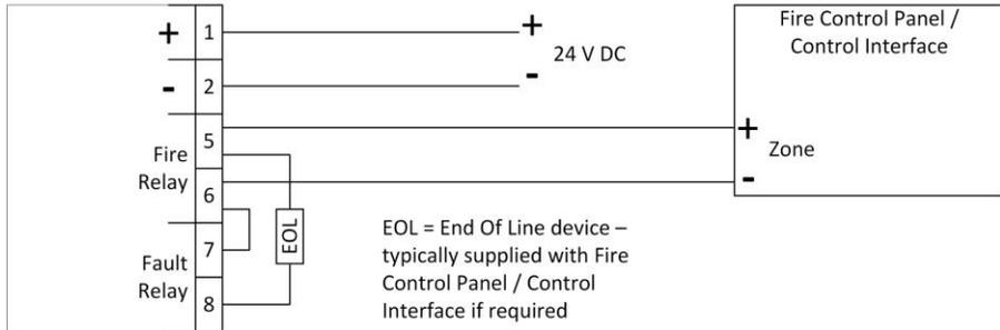
**Fig 7a** 4 Wire Connection Diagram – single detector
