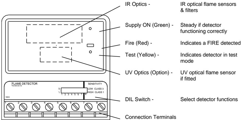
**Fig 4** Detector with Front Cover removed
