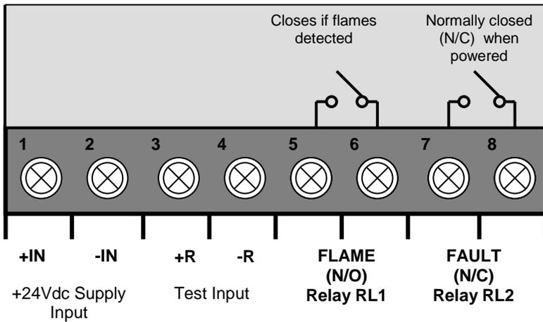
**Fig 3** Electrical Connection Terminals
