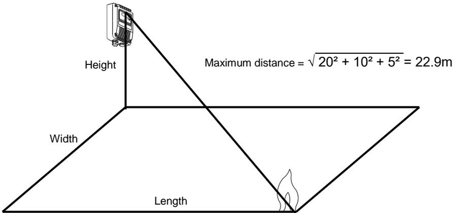
**Fig 1** Calculation of distance from detector to flame
