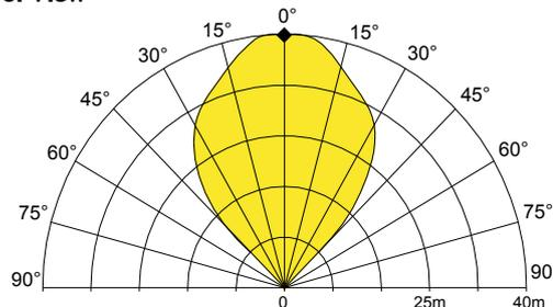
To meet the requirements of EN54:10 clause 5.4, where the ratio of the response points Dmax: Dmin should not exceed 1.41, the horizontal and vertical viewing angles max should not exceed ±30°.
